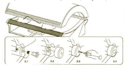
(see fig. 2.2 and 2.3) and cover threadholes with plastic plugs.
