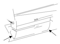
> Lubricate the hinges with HHS2000
